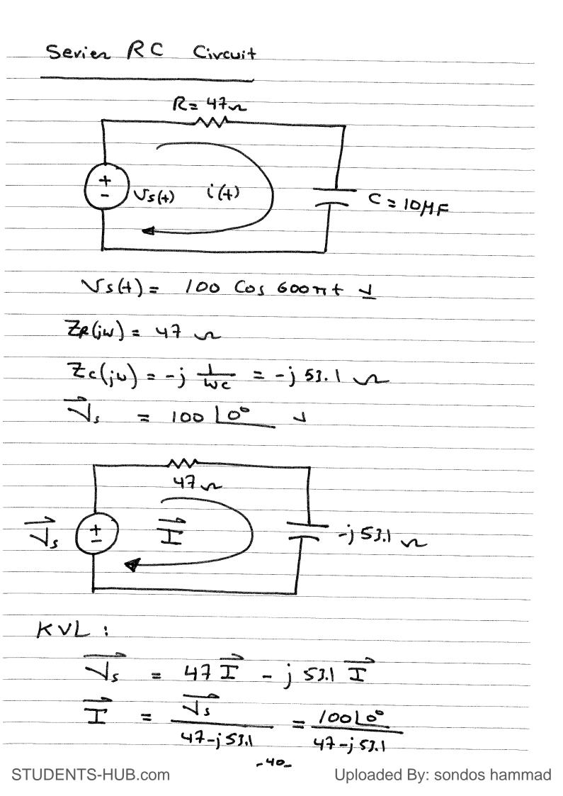
T. 100100 70.91-48.50 T 1.41 248.5° Leads Vs by 48.5° Capacitive Civcuit Z(ju) = 47-j51.1° Capacitive Z(ju) = 70.91-48.5° Capacitive R = 47I = 66.3 48.5° V √c = -j5].1 I = 74.9 [-41.5° V No Lags I by 90° Je 48.50 41.50 41.
