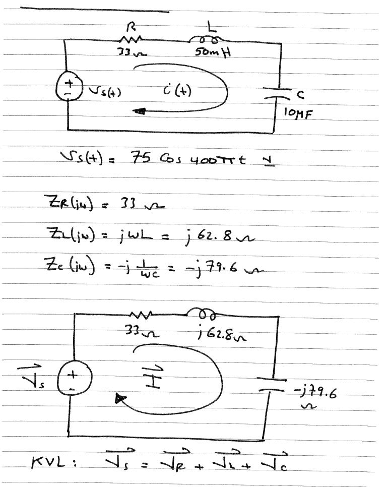
$\sqrt{s} = 33 \vec{T} + j 62.8 \vec{T} - j 79.6 \vec{T}$  $= \frac{\overline{\sqrt{s}}}{\overline{77-j/6.8}}$ 75 l - 220 = 2.03 27° I Leads V5 by 27° Capacitive Civcuit Zeq = R+jWL-j tur Zeq = 3)+j 62.8-j79.6 Zeq = 33- j 16.8 S Capacitive Zeq = 37 [-27° ~ Capacitive  $V_{R} = RI = 67 [27]$ = jWLI = 127 [117°  $c = -j \perp I = 162 \lfloor -63^{\circ} \lor$ -43-
