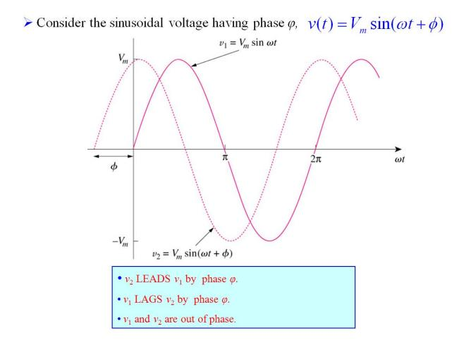
Phase of Sinusoids The terms Lead and Lag are used to indicate the relationship between two sinusoidal wave forms of the same Frequency plotted on the same set of axes Vm sin wt V1(+) =  $V_2(t) = Nm sin (wt+G)$ .: N2(+) Leads V.(+) by G ov VI(+) Lags V2(+) by O -3.
