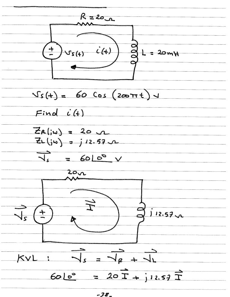
= 60 60 20+ 12.57 23.6 37.10 T = 2.54-32.10  $V_R = 20T = 50.8 [-32.1°$  $L = j_{12.57} T = 31.9 + 57.9^{\circ}$ VI Leads VR by 90° IL Lags Vs by J?.1° Zeq = 20+ j 12.57 ~ inductive = 23.6 ]32.1° ~ inductive 57.90 Phasor diagram - 39 -STUDENTS-HUB.com Uploaded By: sondos hammad
