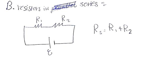
\* procedure :-Powt A : one - resistor, DC - Circuit Avg 6 5 2 4 3 No Mi-R Rh I(m A) V (Vol6) امین = I ۵ نقربر = اکتان = V ۵ Pant B : + Wo-resistors in Series -write down the realings of the Is and Vs only once R2 Ri 3Rn Some DI DN
