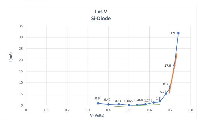
According to the diagram above, which shows the relationship between I and V, it is proved that Si Diode does not obey Ohm's law and it is a nonlinear element.
