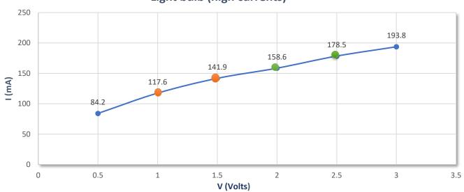
According to the diagram above, which shows the relationship between I and V the light bulb (with high currents) does not obey Ohms and it is a nonlinear element.
