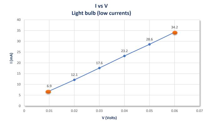
According to the diagram above, which shows the relationship between I and V according to Ohm's law Prove that the light bulb (with low currents) is a linear element.
