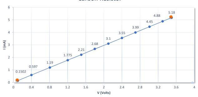
According to the diagram above, which shows the relationship between I and V according to Ohm's law Prove that the carbon resistor is a linear element.
