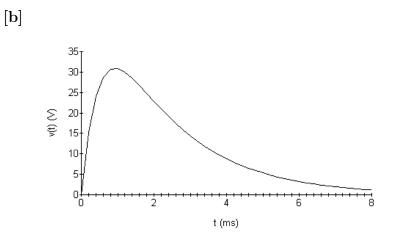
Example 8.4:  $v_{\text{max}} \cong 74.1 \text{ V}$  at 1.4 ms Example 8.5:  $v_{\text{max}} \cong 36.1 \text{ V}$  at 1.0 ms Problem 8.17:  $v_{\text{max}} \cong 30.9$  at 0.92 ms
