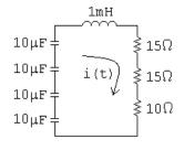
[b]  $s_{1,2} = -\alpha \pm \sqrt{\alpha^2 - \omega_0^2} = -20,000 \pm 0$ Therefore there are two repeated real roots at -20,000 rad/s.
