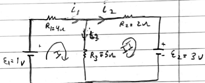
$$\text{for } ①: \epsilon_1 - i_1 R_1 - i_3 R_3 = 0 \quad ③$$
