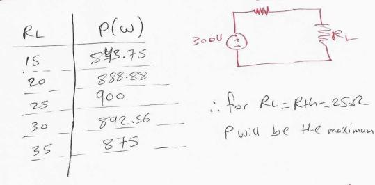
Example 2-Find the Value of RL for maximum power transfer in the airanit shown
