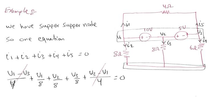
$$\frac{V_{1}}{8} + \frac{V_{2}}{8} + \frac{V_{3}}{8} = 0$$
