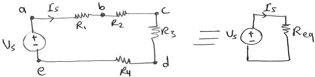
$$R_{eq} = R_1 + R_2 + R_3 + R_4$$
