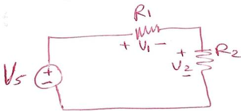
$$V_1 = \frac{V_s R_1}{R_1 + R_2}$$
