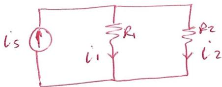
$$i_1 = \frac{i_s R_2}{R_1 + R_2}$$
