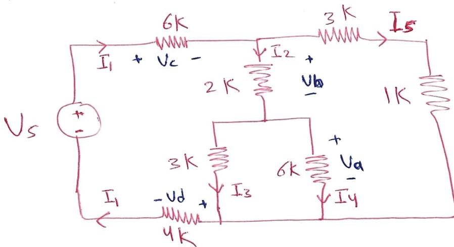
$$V_a = (6\text{K})(0.5\text{mA}) = 3\text{V}$$
