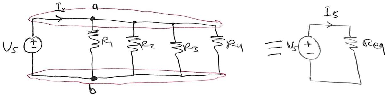
$$\frac{1}{R_{eq}} = \frac{1}{R_1} + \frac{1}{R_2} + \frac{1}{R_3} + \frac{1}{R_4}$$
