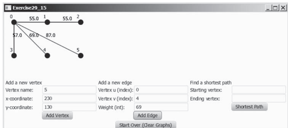
FIGURE 29.27 The program can add vertices and edges and display a shortest path between two specified vertices. Source: Copyright © 1995–2016 Oracle and/or its affiliates. All rights reserved. Used with permission.
