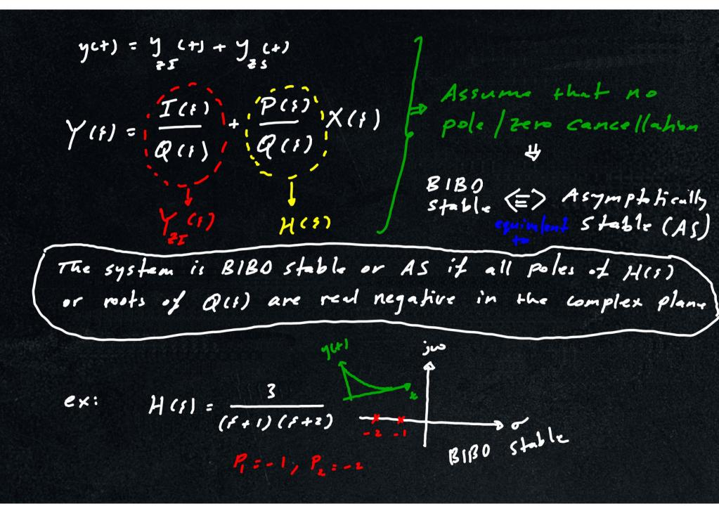
If H(s) has at least one real positive pole or repeated poles with zero real parts, then the system is unstable.
