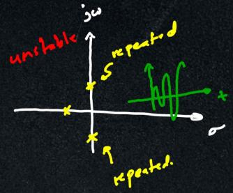
If H(s) has poles (not repeated) and located on the imaginary axis, then the system is marginally stable.
