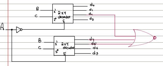
Q4 (10 points): Implement the following function  $F(A,B,C,D) = \sum (0, 2, 4, 6, 8, 10)$ a. Mux 4×1 b. Decoders 3-to-8 c. AND-OR d. NAND-NAND output a) selectors = 2 0 0 ပ 0 O 0 Ø 0 0 1 Ø 0 O F=D b 0 O a 0 O O F=0) O 0 0 0 0 တ a F=0 0 0 l 0 0 0 b) 3-8 decoder В do 3 X 8 d<sub>2</sub> decoder وله with Enable 巨 98 dq 3x8 dio decoder dι with 912 વહ Enable dly
