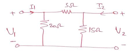
$\begin{aligned} If I_2 &= 0 \\ Z_{11} &= \frac{V_1}{I_1} \Big|_{=} 20 \ 11(5+15) = 10 \ J = 3 \ I_1 = \frac{V_1}{10} \end{aligned}$
