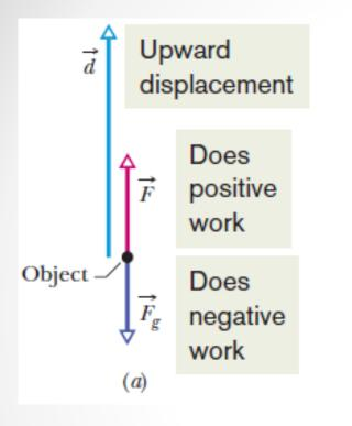
(a) An applied force F lifts an object. The object's displacement  $\vec{d}$  makes an angle  $\phi = 180^{\circ}$  with the gravitational force  $\vec{F_g}$  on the object. The applied force does positive work on the object.
