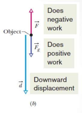
(b) An applied force  $\vec{F}$  lowers an object. The displacement  $\vec{d}$  of the object makes an angle  $\phi = 0^{\circ}$  with the gravitational force  $\vec{F_g}$ . The applied force does negative work on the object.
