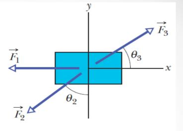
$$F_{\text{net }x} = -F_1 - F_2 \sin 50.0^\circ + F_3 \cos 35.0^\circ = -3.00 \text{ N} - (4.00 \text{ N}) \sin 35.0^\circ + (10.0 \text{ N}) \cos 35.0^\circ = 2.13 \text{ N}$$
