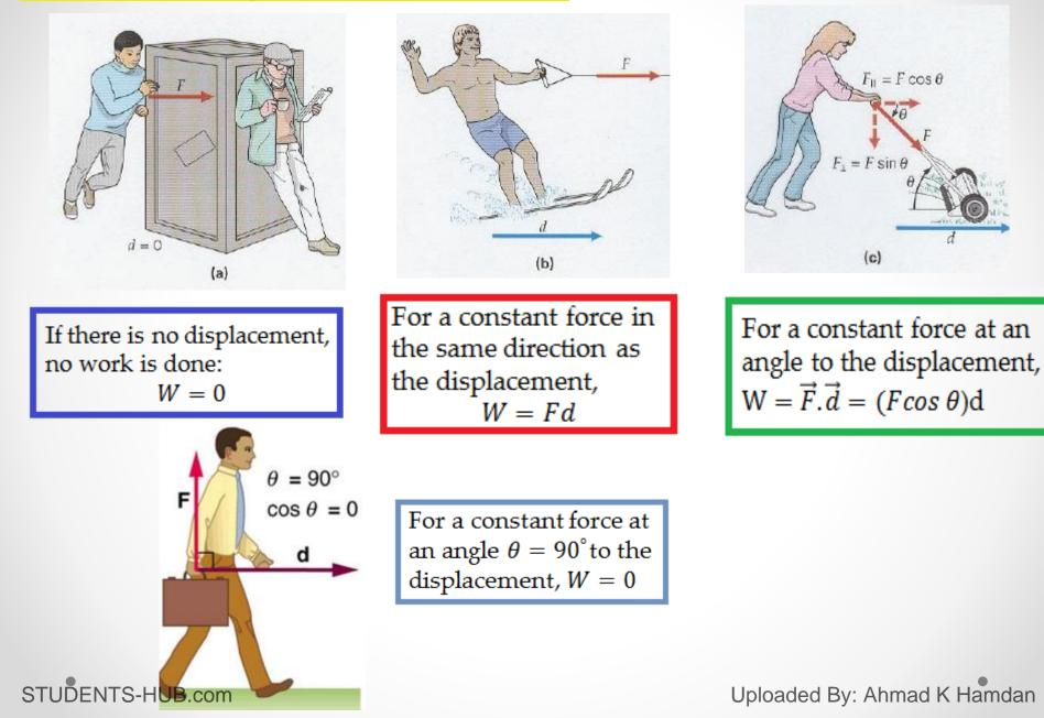
A force does positive work when it has a vector component in the same direction as the displacement, and it does negative work when it has a vector component in the opposite direction. It does zero work when it has no such vector component.
