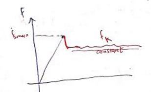
(FSymax = Ms FN), Ms = roffe static Fraction 0 for = Normal Fors
