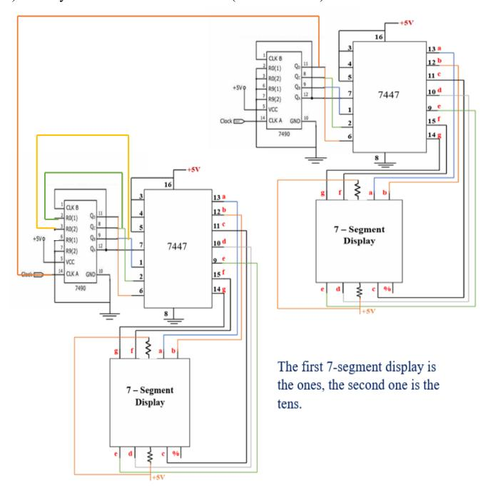
To Modify the counter to count from 00 to 59 then return to 00, the 7-segment that show the tens don't reach 6 (0110). So, we connected pin 8 and 9 ( $Q_CQ_B$ ) to the pin 2 and 3 {R0(1) and R0(2)}, since R0(1) and R0(2) connected with NAND gate then, when the tens display reach 0110 the input of NAND gate is 1,1 and the output of the gate is 0, and the reset work in active low so its return to 0.
