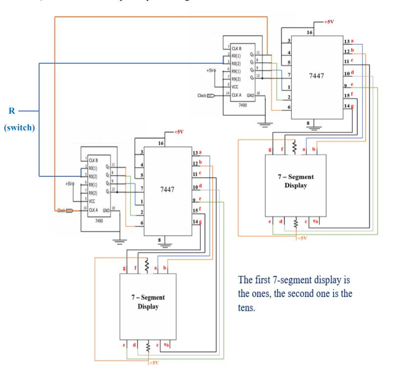
R input: is a switch that work to reset the counter as following:
