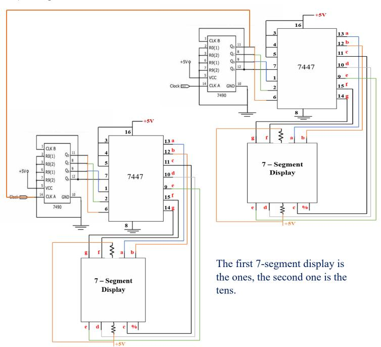
2) Add additional input to your design that can be used to reset the counter.
