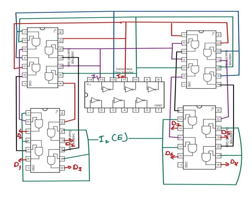
We make  $I_2$  the enable of both decoders, and use  $I_1$  and  $I_0$  as the inputs of the decoders.
