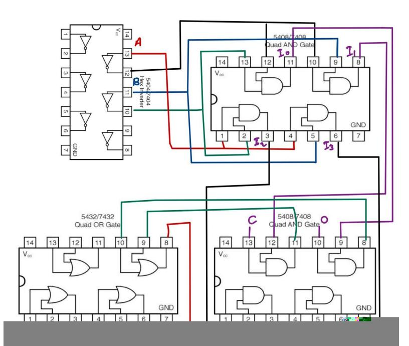
4) Implement f(x, y, z) = m(0, 1, 4, 6, 7), using 4x1 MUX using chips in Figure 1.
