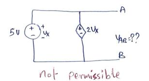
Connecting Current sources parallel Current sources add together while series current sources should have the same value and direction. Nove the same value and direction. SA () SA () Not permissible STUDENTS-HUB.compa
