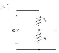
Maximum dissipation in  $R_2$  occurs at no load, therefore,
