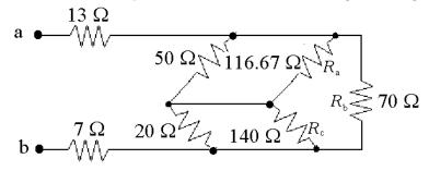
Find the equivalent resistance to the right of the  $13\,\Omega$  and  $7\,\Omega$  resistors:
