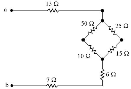
Replace the  $\Delta$  with its equivalent Y in the circuit to get the figure below:
