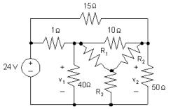
Now use Eqs. 3.44 - 3.46 to calculate the values of the Y-connected resistors:
