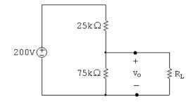
[a] We can use voltage division to calculate the voltage  $v_o$  across the 75 k $\Omega$  resistor:
