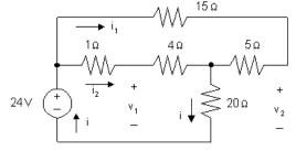
The equivalent resistance seen by the 24 V source can be calculated by making series and parallel combinations of the resistors to the right of the 24 V source:
