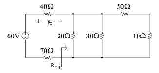
[a] First we need to determine the equivalent resistance to the right of the  $40 \Omega$  and  $70 \Omega$  resistors:
