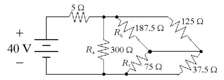
Find the equivalent resistance to the right of the  $5\,\Omega$  resistor:
