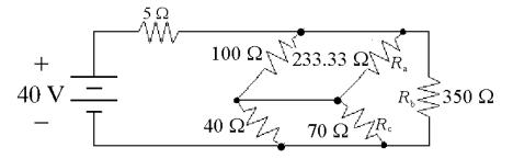
Find the equivalent resistance to the right of the  $5\,\Omega$  resistor:
