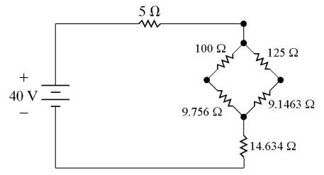
Find the equivalent resistance to the right of the  $5\,\Omega$  resistor:
