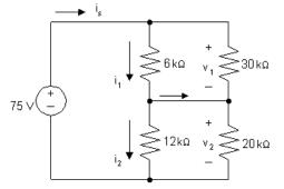
$6 \text{ k}\Omega \parallel 30 \text{ k}\Omega = 5 \text{ k}\Omega$
