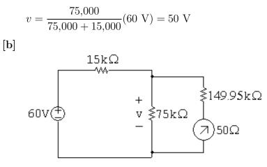
The meter resistance is a series combination of resistances:
