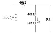
[a] We will write a current division equation for the current throught the  $80\Omega$  resistor and use this equation to solve for R:
