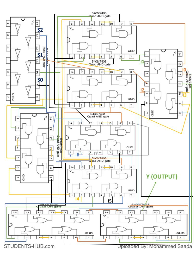
e) Use the just constructed 4x1 multiplexer to design a three input network that gives 1 if the majority of its input are 1 and output a zero otherwise.
