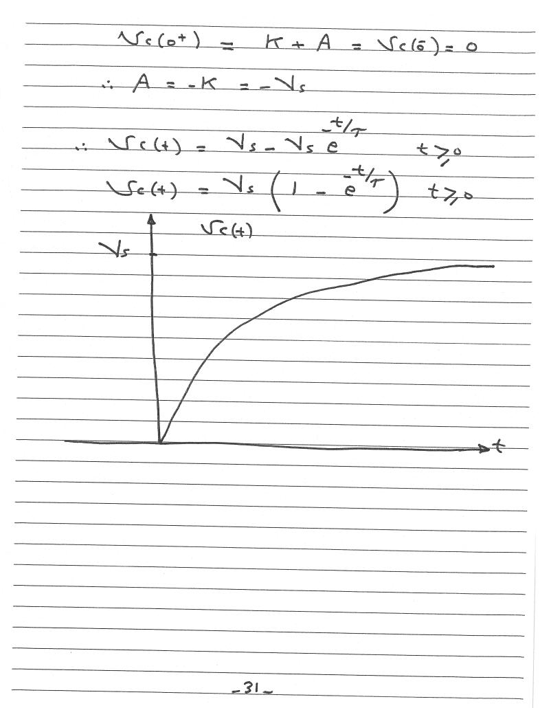
When all independent sources are Constant, the response of the First order Circuit has the form V(t) = Vn(t) + K $V(t) = Ae^{\tau} + K \qquad t > 0$ Y (&) : V(+) = Ae + V(00) +>0 V (ot) = A + V (cs)  $A = V(\delta) - V(\delta)$ :  $V(+) = V(\infty) + [V(0^{+}) - V(\infty)] e^{-t/2}$ TERESCE
