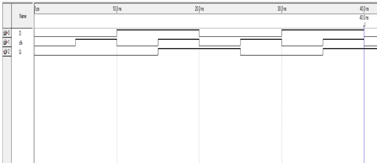
Figure 2. 6 : D - Flip Flop - Waveform
