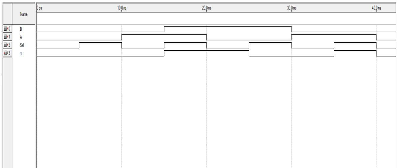
Figure 2. 8 : 2x1 MUX – Waveform
