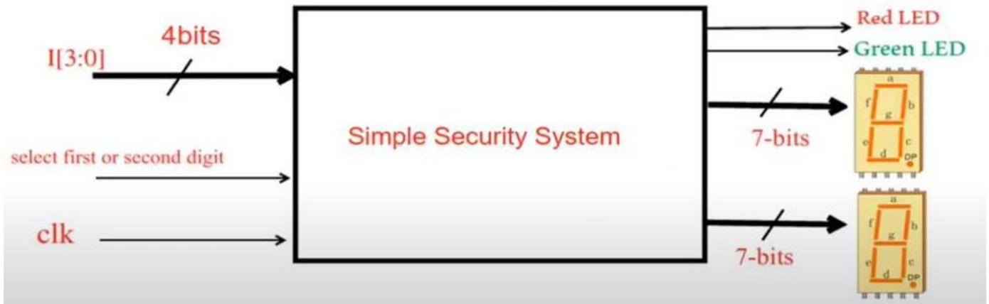
Figure 2 : High level view of the system (Source : Lab Manual)
