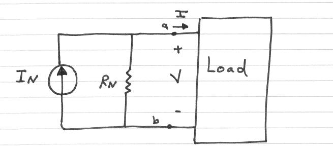
It states that a Linear two terminal Circuit Can be replaced by an equivalent Circuit of a current source In in parellel With a resistor RN.
