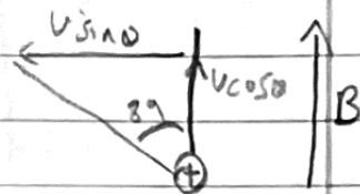
$$\text{but } r = \frac{mv \sin \phi}{eB} \quad (\text{helical path})$$
