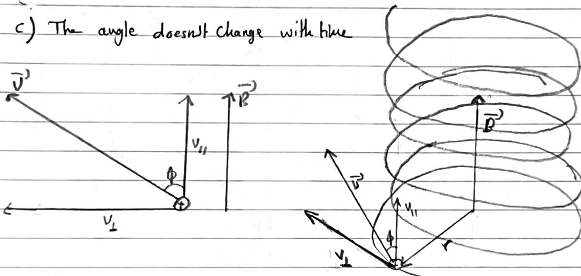
$$d) F_B = F_c \Rightarrow v_{\perp} = v \sin \phi$$
