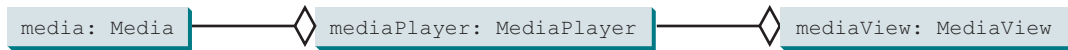
FIGURE 16.34 The media represents the source, the media player controls the playing, and the media view displays the video.
