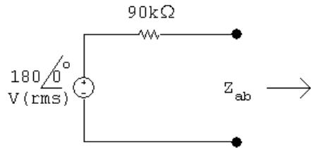
For maximum power transfer,  $Z_{ab} = 90 \text{ k}\Omega$
