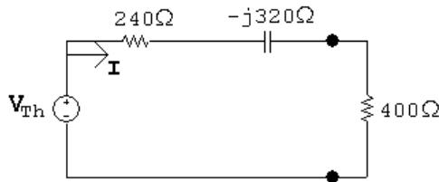
$$\mathbf{I} = \frac{60 + j60}{640 - j320} = 37.5 + j112.5 \text{ mA(rms)} = 118.59/\underline{71.57^\circ} \text{ mA(rms)}$$
