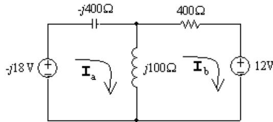
$$\mathbf{I}_a = 67.5 - j7.5 \text{ mA} \quad \text{and} \quad \mathbf{I}_b = -22.5 + j22.5 \text{ mA}$$
