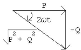
$$\cos 2\omega t = \frac{P}{\sqrt{P^2 + Q^2}}; \quad \sin 2\omega t = -\frac{Q}{\sqrt{P^2 + Q^2}}$$
