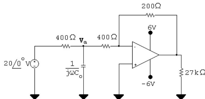
$$\frac{\mathbf{V}_a - 20\angle0^\circ}{400} + j\omega C_o \mathbf{V}_a + \frac{\mathbf{V}_a}{400} = 0$$
