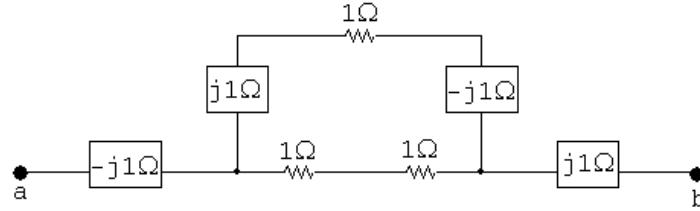
Simplify the middle portion of the circuit by making series and parallel combinations:
