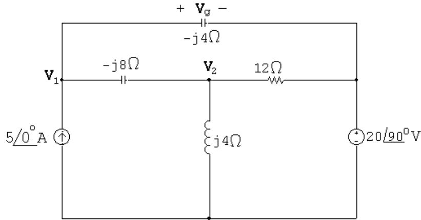
$$\text{At } \mathbf{V}_1: \quad -5\angle 0^\circ + \frac{\mathbf{V}_1 - \mathbf{V}_2}{-j8} + \frac{\mathbf{V}_1 - 20\angle 90^\circ}{-j4} = 0$$
