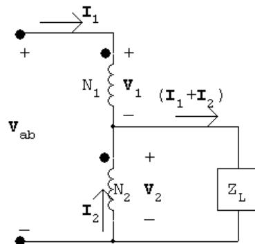
$$Z_{ab} = \frac{V_{ab}}{I_1} = \frac{V_1 + V_2}{I_1}$$
