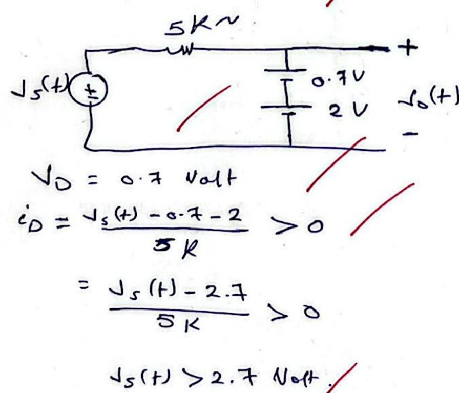
:. When  $V_s(t) > 2.7 \text{ Volt}$ the Diode is on  $J_D = 0.7 \text{ Volt}$ .  $J_0(t) = 0.7 + 2$ = 2-7 Volt.
