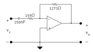
[b] The passband gain changes but the cutoff frequency is unchanged.
