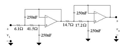
P 15.43 [a] The cascade connection is a bandpass filter.
