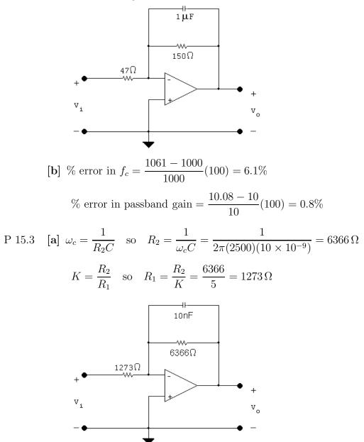
[b] Both the cutoff frequency and the passband gain are changed.
