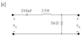
P 15.16 [a] Since  $\omega_o^2 = 1/LC$  and  $\omega_o = 1$  rad/s,  $C = \frac{1}{L} = \frac{1}{Q}$  F [b]  $H(s) = \frac{(R/L)s}{s^2 + (R/L)s + (1/LC)}$
