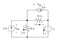
[a] To find  $v_s$ , write a KVL equation, summing the voltages counter-clockwise around the lower right loop. Start below the voltage source.
