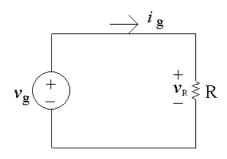
[a] The resistor and the voltage source are in parallel and the resistor voltage and the voltage source have the same polarities. Therefore these two voltages are the same:
