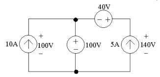
From the values of voltage and current in the figure, the power supplied by the current sources is calculated as follows:
