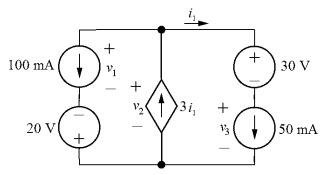
The voltage drop across the left branch, the center branch, and the right branch must be the same, since these branches are connected at the same two terminals. This requires that
