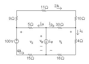
$$v_2 = 100 + 4(15) = 160 \text{ V};$$
