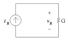
[a] Note from the circuit that the current through the conductance G is  $i_g$ , flowing from top to bottom, because the current source and the
