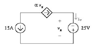
[a] Note from the circuit that  $v_x = -25$  V. To find  $\alpha$  note that the two current sources are in the same branch of the circuit but their currents flow in opposite directions. Therefore
