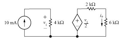
$$v_1 = (4000)(0.01) = 40 \,\text{V}$$
