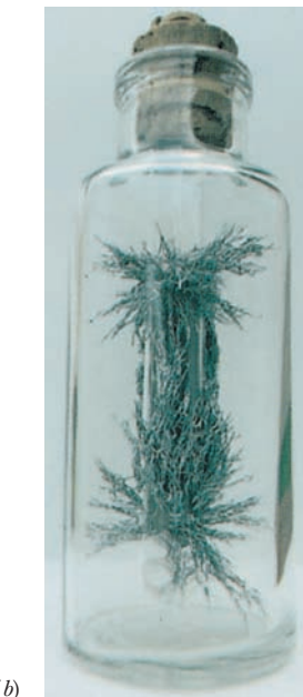
Figure 28-4 (a) The magnetic field lines for a bar magnet. (b) A “cow magnet”—a bar magnet that is intended to be slipped down into the rumen of a cow to prevent accidentally ingested bits of scrap iron from reaching the cow's intestines. The iron filings at its ends reveal the magnetic field lines.
