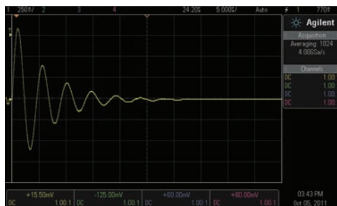
Figure 31-3 An oscilloscope trace showing how the oscillations in an RLC circuit actually die away because energy is dissipated in the resistor as thermal energy.
