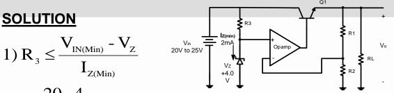
$$R_3 \le \frac{20-4}{2 \text{ mA}} = 8 \text{ k}\Omega$$
