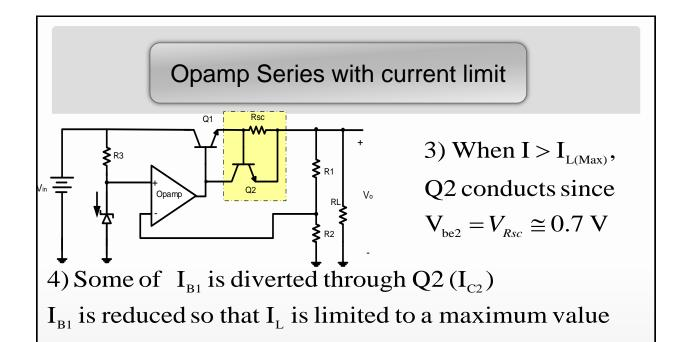
calculated as:  $I_{L(Max)} = \frac{V_{be}}{R_{SC}} = \frac{0.7 \text{ V}}{R_{SC}}$ 5) Since  $V_{be2}$  cannot exceed 0.7 V,  $V_{R_{SC}}$  is limited
