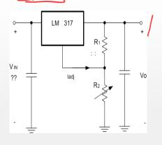
$V_0 = I_{REF}(R_1 + R_2) + I_{Adj}(R_2)$   $I_{REF} = I_{R_1} = \frac{1.25}{220} = 5.68 \text{mA}$ ;  $I_{Adj} = 50 \mu \text{A}$   $V_0 = 5.68 \text{ mA} (220 + 5 \text{K}) + 50 \mu \text{ X} 5 \text{K} = 29.91 \text{ V}$
