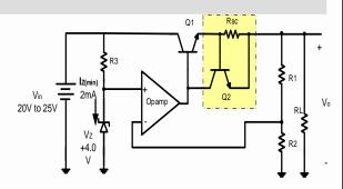
2) — The change for current limit is done by adding Q2 and Rsc as shown
