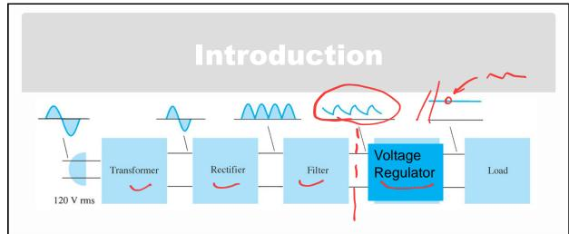
Regulator. a circuit used to produces a constant dc output voltage by reducing the ripple to negligible amount regardless of variation of input voltage and load within reasonable limits
