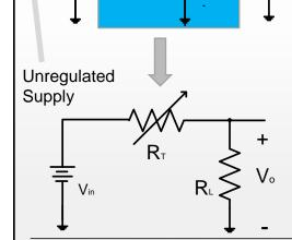
The Transistor behaves like a simple variable resistor whose resistance is determined by the operating conditions
