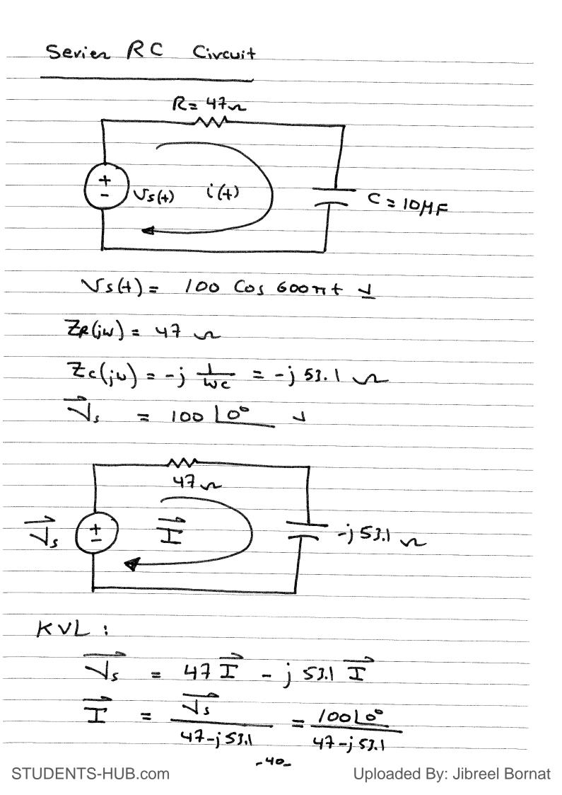
T. 100100 70.91-48.50 T 1.41 248.50 Leads Vs by 48.5° Capacitive Civcuit Z(ju) = 47-j51.1° Capacitive Z(ju) = 70.91-48.5° Cfacitive R = 47I = 66.3 48.5° V √c = -j5].1 I = 74.9 [-41.5° V No Lags I by 90° JR 48.50 41.50 41\_
