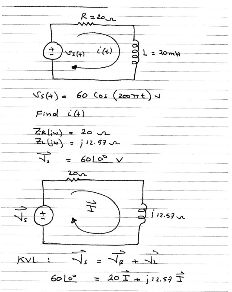
= 60 60 20+ 12.57 23.6 37.10 T = 2.54-32.10  $V_R = 20T = 50.8 [-32.1°$  $L = j_{12.57} I = 31.9 + 57.9^{\circ}$ Leads NR by 90° IL Lags Vs by J?.1° Zeq = 20+ j 12.57 ~ inductive = 23.6 ]32.1° ~ inductive 57.90 Phasor diagram - 39 -STUDENTS-HUB.com
