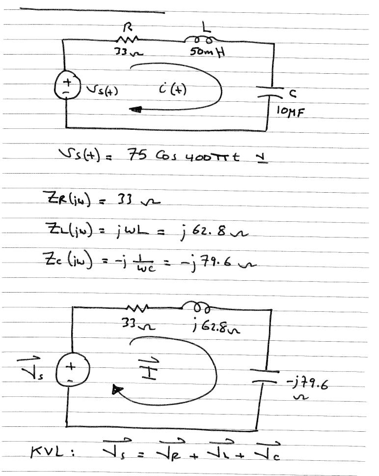
$\sqrt{s} = 33 \vec{T} + j 62.8 \vec{T} - j 79.6 \vec{T}$  $= \frac{\overline{\sqrt{s}}}{\overline{77-j}}$ 75 l - 270 = 2.03 27° I Leads V5 by 27° Capacitive Civcuit Zeq = R+jWL-j tur Zeq = 3)+j 62.8-j79.6 Zeq = 33- j 16.8 S Capacitive Zeq = 37 [-27° ~ Capacitive  $V_{R} = RI = 67 [27]$ 1130 = jWLI = 1271  $c = -j \perp I = 162 \lfloor -63^{\circ} \lor$ -43-
