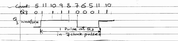
e. With a clock frequency of 1400 pulses per second, the signal at output Q3 of the counter has a frequency of 200 pulses per second.
