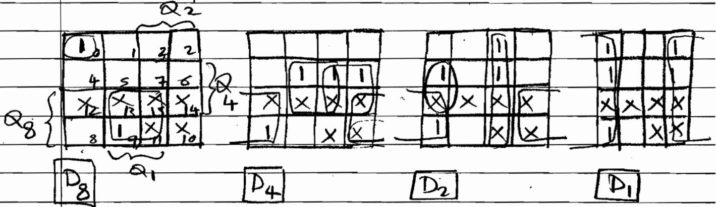
$$D_8 = Q_1 \bar{Q}_2 + \bar{Q}_1 \bar{Q}_2 \bar{Q}_4 \bar{Q}_8$$
