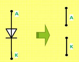
▶ When  $V_s < V_o$ ; the Diode is off, and replaced with open circuit
