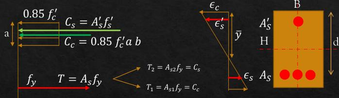
$\overline{\phi M_{n_1}} = \overline{\phi A_s' f_y} (d - \underline{d'})$
