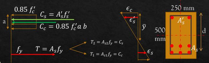
assume 2 layers of steel in bottom  $d = 417 \text{ mm } \dots d' = 60 \text{ mm}$
