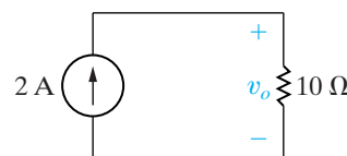
Figure 4.43 ▲ The circuit shown in Fig. 4.42 after combining sources and resistors.
