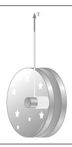
By pulling on the string of a yo-yo, a person manages to make the yo-yo spin, while remaining at the same elevation above the floor. Denoting the mass of the yo-yo by m, the radius of the inner drum on which the string is wound by r, and the centroidal radius of gyration of the yo-yo by  $\overline{k}$ , determine the angular acceleration of the yo-yo.
