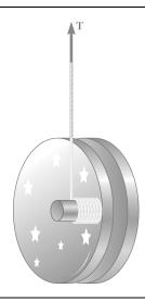
The 80-g yo-yo shown has a centroidal radius of gyration of 30 mm. The radius of the inner drum on which a string is wound is 6 mm. Knowing that at the instant shown the acceleration of the center of the yo-yo is  $1 \text{ m/s}^2$  upward, determine (a) the required tension **T** in the string, (b) the corresponding angular acceleration of the yo-yo.
