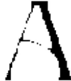
Erosion by 5*5 square structuring element
