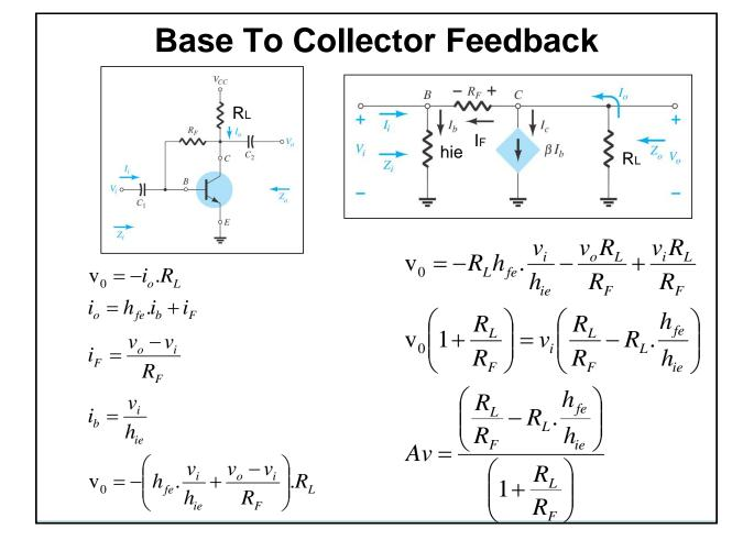
$$Z_{0}\Big|_{v_{i}=0} = R_{F} // R_{L}$$
