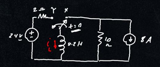
The switch is set in position x for a long time. At top, the switch moves to position Y.
