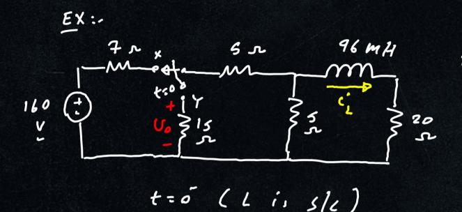
The switch hav been in position X for a long time. At t=0, the switch moves to position Y. Find Uo(4) ty, 0.
