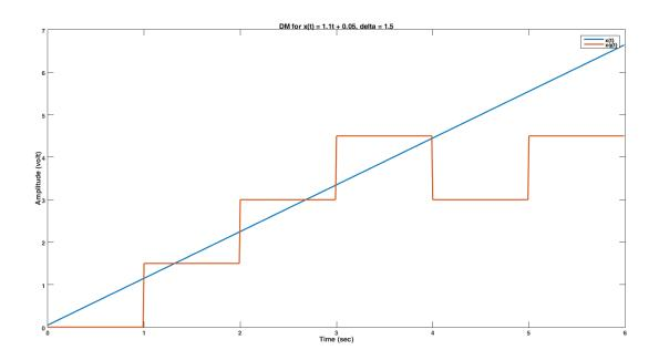
The plots above show that when  $\Delta = 1$ , the DM output is the closest to the original signal, where when  $\Delta = 0.5$  the output doesn't follow closely the actual curve, which makes slope overload distortion. Also increasing  $\Delta$  to 1.5 makes higher granular noise to the output.
