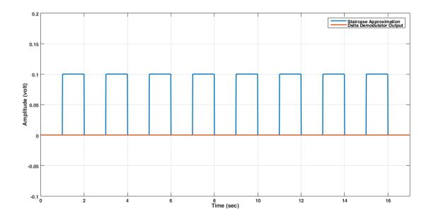
It's noticed that the staircase approximation is a square wave which can't be used to approximate the original signal due to wide sampling period  $T_S$ . The output of a delta demodulator will be zero due to low-pass filtering for the oscillating.
