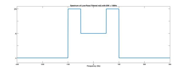
c) There is a distortion due to aliasing occurred by sampling process which is noticed in the spectrum of sampled signal. Also it can be noticed that the spectrum of the signal after applying to a low-pass filter with bandwidth of 100Hz is not identical to the original spectrum.
