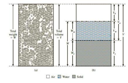
$V = V_{x} + V_{y} = V_{x} + V_{y} + V_{y}$
