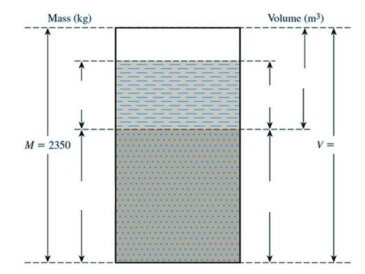
• Relative density  $(D_r)$ : commonly used to indicate the in-situ denseness or looseness of granular soil
