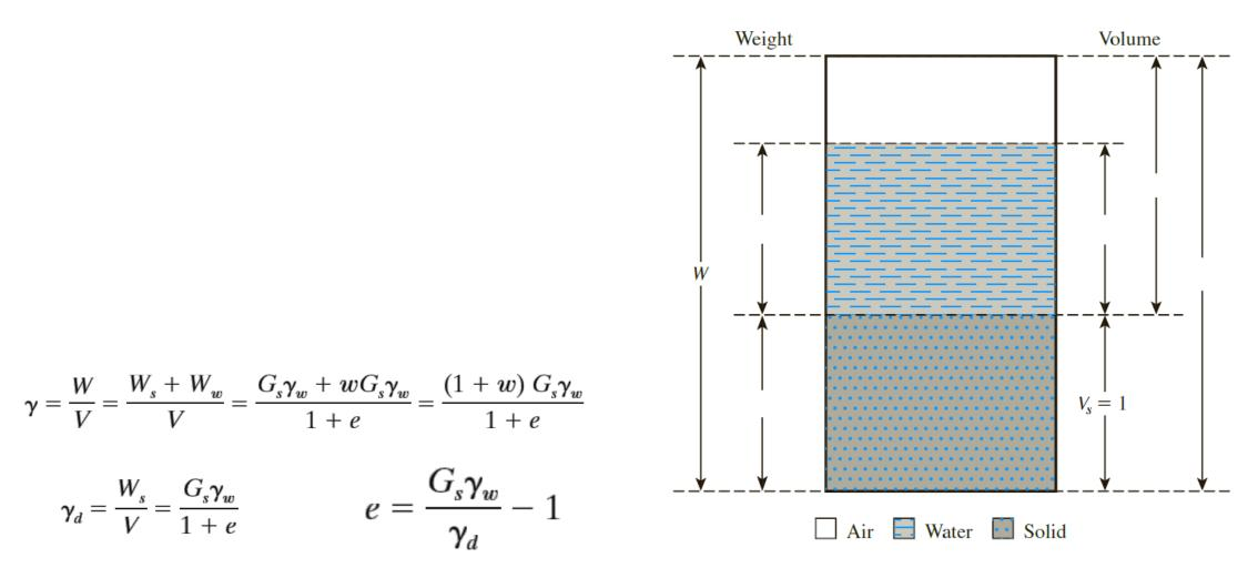
• Relationships among Unit Weight, Void Ratio, Moisture Content, and Specific Gravity of soil solids
