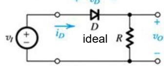
A) when  $V_i(t) > 0$ , Diode is on (short circuit)
