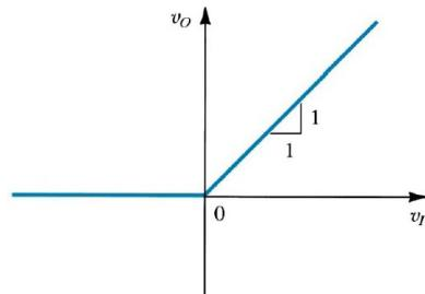
Design a diode circuit that have the given characteristic curve
