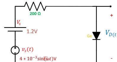
Since we have a dc source (1.2 V) and an ac signal ( $4 \times 10^{-3} \sin(\omega t)$  V) and the diode is always on ; we use superposition theorem to find  $V_D(t)$
