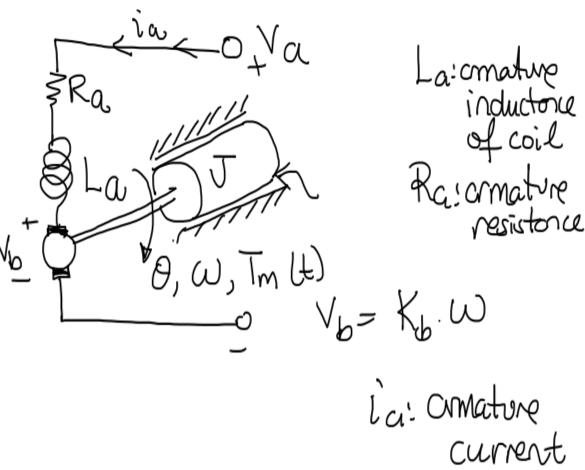
If it is constant, we have on amother controlled DC motor. The torque [In (t) is given by
