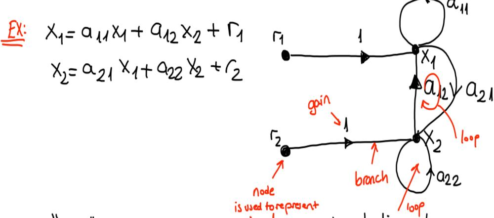
· A Loop is a closed path terminating at the storting node.
