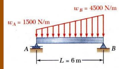
A beam supports a distributed load as shown. Determine the equivalent concentrated load and the reactions at the supports.
