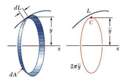
• Area of a surface of revolution is equal to the length of the generating curve times the distance traveled by the centroid through the rotation.
