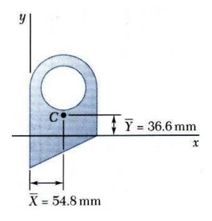
$$\overline{X} = \frac{\sum \overline{x}A}{\sum A} = \frac{+757.7 \times 10^3 \,\text{mm}^3}{13.828 \times 10^3 \,\text{mm}^2}$$
