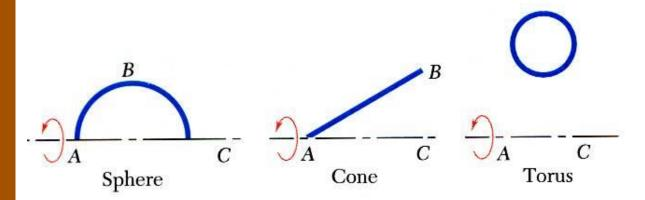
• Surface of revolution is generated by rotating a plane curve about a fixed axis.
