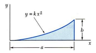
Determine by direct integration the location of the centroid of a parabolic spandrel.
