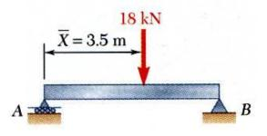
• Determine the support reactions by summing moments about the beam ends.
