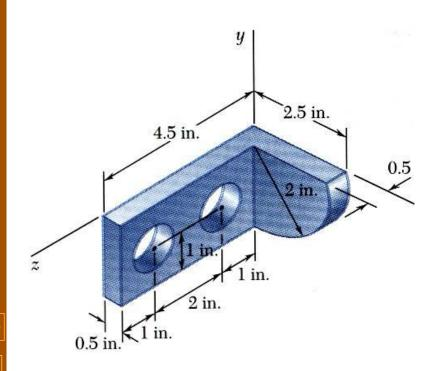
Locate the center of gravity of the steel machine element. The diameter of each hole is 1 in.
