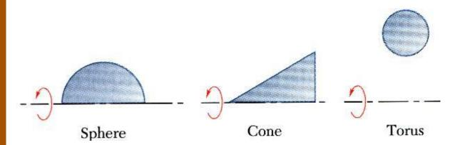
• Body of revolution is generated by rotating a plane area about a fixed axis.
