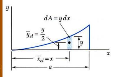
$$Q_y = \int \overline{x}_{el} dA = \int xy dx = \int_0^a x \left(\frac{b}{a^2} x^2\right) dx$$
