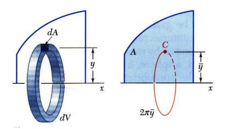
• Volume of a body of revolution is equal to the generating area times the distance traveled by the centroid through the rotation.
