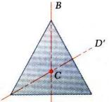
• The first moment of an area with respect to a line of symmetry is zero.
