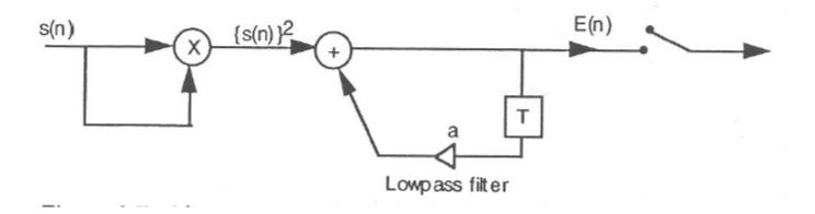
The quantity E(n) must be computed at each sample of input speech signal, even though a much lower sampling rate suffice.
