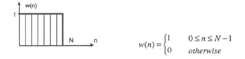
$$W(z) = \sum_{n=0}^{N-1} w(n) z^{-n} = 1 + z^{-1} + z^{-2} + z^{-3} + \dots + z^{-(N-1)} = \frac{1 - z^{-N}}{1 - z^{-1}}$$
