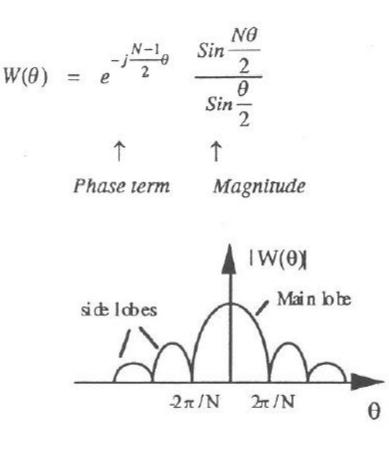
If N is too small,  $E_m$  will fluctuate very rapidly depending on exact details of the waveform.
