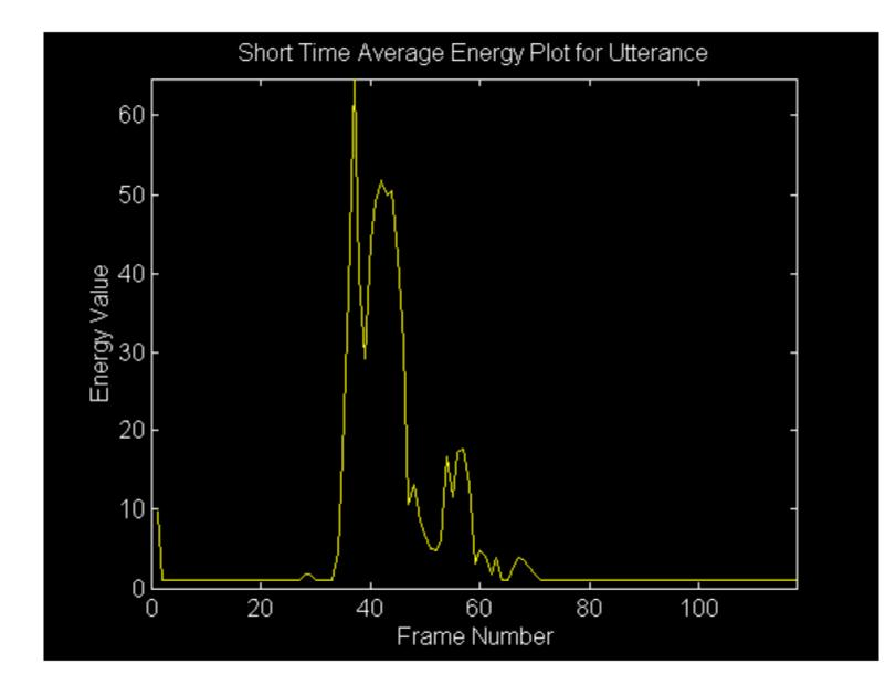
Note that a recursive lowpass filter H(z) can also be used to calculate the short-time energy:
