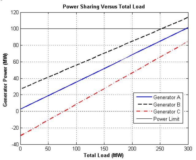
This plot reveals that there are power sharing problems both for high loads and for low loads. Generator B is the first to exceed its ratings as load increases. Its rated power is reached at a total load of 253 MW. On the other hand, Generator C gets into trouble as the total load is reduced. When the total load drops to **STUDENTS-HUB.com** 78 MW, the direction of power flow reverses in Generator C.
