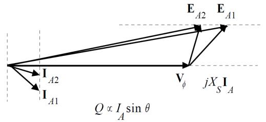
$$P = \frac{3V_{\phi}E_A}{X_s}\sin\delta = \text{constant}, \text{ so } E_{A1}\sin\delta_1 = E_{A2}\sin\delta_2$$
