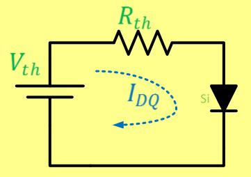
since  $V_{th} \ge V_k$ , the diode is on
