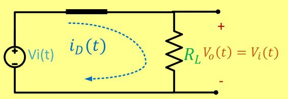
$\therefore$  when  $V_i(t) > 0$ , the diode is on and  $V_O(t) = V_i(t)$ students  $V_0(t) = 0$ , the diode is off and  $V_O(t) = ?$
