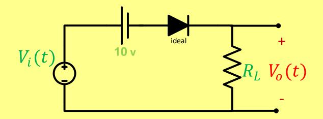
$\therefore$  when  $V_i(t) > 10$  V, the diode is on and  $V_O(t) = V_i - 10$
