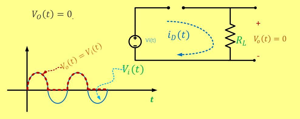
$\therefore$  the clipper circuit used to eliminate portion of the input signal .
