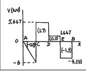
$|V|_{\text{max}} = 6 \text{ kN} \triangleleft$
