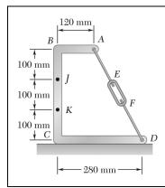
Knowing that the turnbuckle has been tightened until the tension in wire AD is 850 N, determine the internal forces at point indicated:
