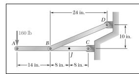
Determine the internal forces (axial force, shearing force, and bending moment) at Point J of the structure indicated.
