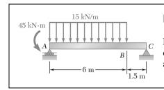
For the beam and loading shown, (a) draw the shear and bending-moment diagrams, (b) determine the magnitude and location of the maximum absolute value of the bending moment.
