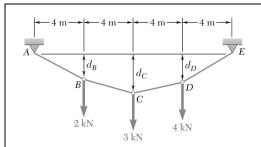
Three loads are suspended as shown from the cable *ABCDE*. Knowing that  $d_C = 3$  m, determine (a) the components of the reaction at E, (b) the maximum tension in the cable.
