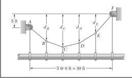
An oil pipeline is supported at 6-ft intervals by vertical hangers attached to the cable shown. Due to the combined weight of the pipe and its contents the tension in each hanger is 400 lb. Knowing that  $d_C = 12$  ft, determine (a) the maximum tension in the cable, (b) the distance  $d_D$ .
