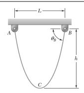
A 10-ft rope is attached to two supports A and B as shown. Determine (a) the span of the rope for which the span is equal to the sag, (b) the corresponding angle  $\theta_B$ .
