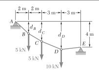
Knowing that  $d_C = 3$  m, determine (a) the distances  $d_B$  and  $d_D$  (b) the reaction at E.
