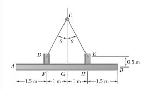
Two small channel sections DF and EH have been welded to the uniform beam AB of weight W=3 kN to form the rigid structural member shown. This member is being lifted by two cables attached at D and E. Knowing that  $\theta=30^{\circ}$  and neglecting the weight of the channel sections, (a) draw the shear and bending-moment diagrams for beam AB, (b) determine the maximum absolute values of the shear and bending moment in the beam.
