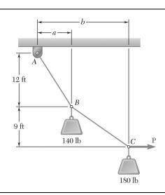
Cable ABC supports two loads as shown. Knowing that b = 21 ft, determine (a) the required magnitude of the horizontal force **P**, (b) the corresponding distance a.
