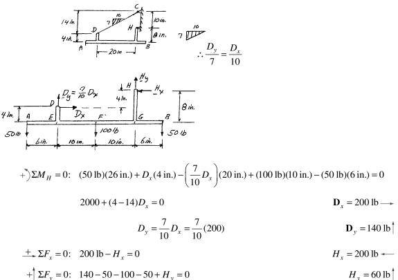
Equivalent loading on straight part of beam AB.
