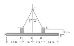
For the structural member of Problem 7.53, determine (a) the angle  $\theta$  for which the maximum absolute value of the bending moment in beam AB is as small as possible, (b) the corresponding value of  $|M|_{\text{max}}$ . (Hint: Draw the bending-moment diagram and then equate the absolute values of the largest positive and negative bending moments obtained.)
