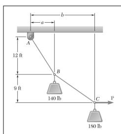
Cable ABC supports two loads as shown. Determine the distances a and b when a horizontal force  $\mathbf{P}$  of magnitude 200 lb is applied at A.
