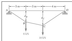
Two loads are suspended as shown from the cable *ABCD*. Knowing that  $d_B = 1.8$  m, determine (a) the distance  $d_C$ , (b) the components of the reaction at D, (c) the maximum tension in the cable.
