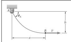
A uniform cable weighing 3 lb/ft is held in the position shown by a horizontal force **P** applied at *B*. Knowing that P = 180 lb and  $\theta_A = 60^\circ$ , determine (*a*) the location of Point *B*, (*b*) the length of the cable.
