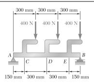
Draw the shear and bending-moment diagrams for the beam AB, and determine the maximum absolute values of the shear and bending moment.
