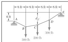
If  $d_C = 8$  ft, determine (a) the reaction at A, (b) the reaction at E.
