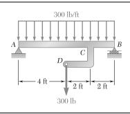
Solve Problem 7.83 assuming that the 300-lb force applied at D is directed upward.
