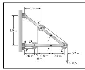
Knowing that the radius of each pulley is 200 mm and neglecting friction, determine the internal forces at Point K of the frame shown.
