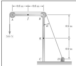
Knowing that the radius of each pulley is 150 mm, that  $\alpha = 20^{\circ}$ , and neglecting friction, determine the internal forces at (a) Point J, (b) Point K.
