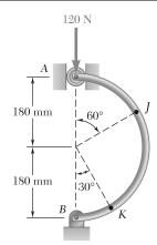
A semicircular rod is loaded as shown. Determine the internal forces at Point *K*.
