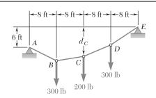
If  $d_C = 4.5$  ft, determine (a) the reaction at A, (b) the reaction at E.
