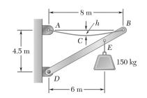
The total mass of cable ACB is 20 kg. Assuming that the mass of the cable is distributed uniformly along the horizontal, determine (a) the sag h, (b) the slope of the cable at A.
