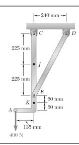
Determine the internal forces at Point *K* of the structure shown.
