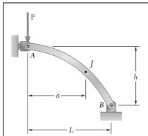
The axis of the curved member AB is a parabola with vertex at A. If a vertical load **P** of magnitude 450 lb is applied at A, determine the internal forces at J when h = 12 in., L = 40 in., and a = 24 in.
