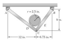
For the frame of Problem 7.17, determine the magnitude and location of the maximum bending moment in member BC.
