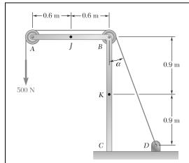
Knowing that the radius of each pulley is 150 mm, that  $\alpha = 30^{\circ}$ , and neglecting friction, determine the internal forces at (a) Point J, (b) Point K.
