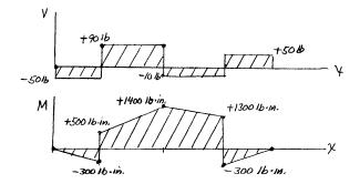
$$|V|_{\text{max}} = 90.0 \text{ lb}; \quad |M|_{\text{max}} = 1400 \text{ lb} \cdot \text{in.} \blacktriangleleft$$
