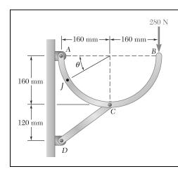
A semicircular rod is loaded as shown. Determine the internal forces at Point *J* knowing that  $\theta = 30^{\circ}$ .
