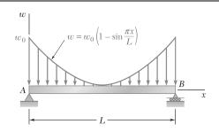
For the beam and loading shown, (a) write the equations of the shear and bending-moment curves, (b) determine the maximum bending moment.
