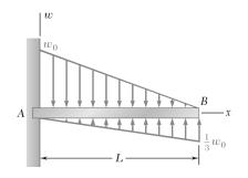
For the beam and loading shown, (a) write the equations of the shear and bending-moment curves, (b) determine the magnitude and location of the maximum bending moment.
