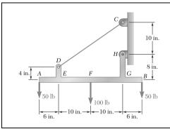
Draw the shear and bending-moment diagrams for the beam AB, and determine the maximum absolute values of the shear and bending moment.
