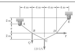
If a = 4 m, determine the magnitudes of **P** and **Q** required to maintain the cable in the shape shown.
