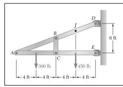
Determine the internal forces (axial force, shearing force, and bending moment) at Point J of the structure indicated.
