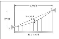
Each cable of the side spans of the Golden Gate Bridge supports a load w = 10.2 kips/ft along the horizontal. Knowing that for the side spans the maximum vertical distance h from each cable to the chord AB is 30 ft and occurs at midspan, determine (a) the maximum tension in each cable, (b) the slope at B.
