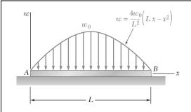
The beam AB, which lies on the ground, supports the parabolic load shown. Assuming the upward reaction of the ground to be uniformly distributed, (a) write the equations of the shear and bending-moment curves, (b) determine the maximum bending moment.
