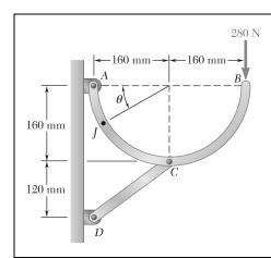
A semicircular rod is loaded as shown. Determine the magnitude and location of the maximum bending moment in the rod.
