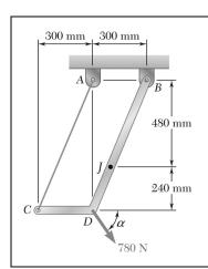
Determine the internal forces at Point J when  $\alpha = 90^{\circ}$ .
