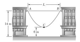
A 40-m cable is strung as shown between two buildings. The maximum tension is found to be 350 N, and the lowest point of the cable is observed to be 6 m above the ground. Determine (a) the horizontal distance between the buildings, (b) the total mass of the cable.
