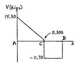
$|V|_{\text{max}} = 15.30 \text{ kips} \blacktriangleleft$ (*b*)
