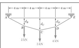
Knowing that the maximum tension in cable *ABCDE* is 13 kN, determine the distance  $d_C$ .
