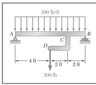
(a) Draw the shear and bending-moment diagrams for beam AB, (b) determine the magnitude and location of the maximum absolute value of the bending moment.
