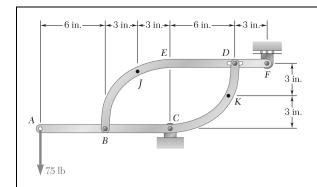
Two members, each consisting of a straight and a quarter-circular portion of rod, are connected as shown and support a 75-lb load at A. Determine the internal forces at Point J.
