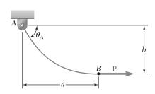
A uniform cable weighing 3 lb/ft is held in the position shown by a horizontal force **P** applied at *B*. Knowing that P = 150 lb and  $\theta_A = 60^\circ$ , determine (a) the location of Point B, (b) the length of the cable.
