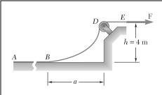
To the left of Point B the long cable ABDE rests on the rough horizontal surface shown. Knowing that the mass per unit length of the cable is 2 kg/m, determine the force F when a = 6 m.
