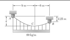
Cable ACB supports a load uniformly distributed along the horizontal as shown. The lowest Point C is located 9 m to the right of A. Determine (a) the vertical distance a, (b) the length of the cable, (c) the components of the reaction at A.
