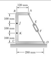
Knowing that the turnbuckle has been tightened until the tension in wire AD is 850 N, determine the internal forces at point indicated:
