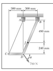
Determine the internal forces at Point J when  $\alpha = 0$ .
