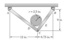
A 5-in.-diameter pipe is supported every 9 ft by a small frame consisting of two members as shown. Knowing that the combined weight of the pipe and its contents is 10 lb/ft and neglecting the effect of friction, determine the magnitude and location of the maximum bending moment in member AC.
