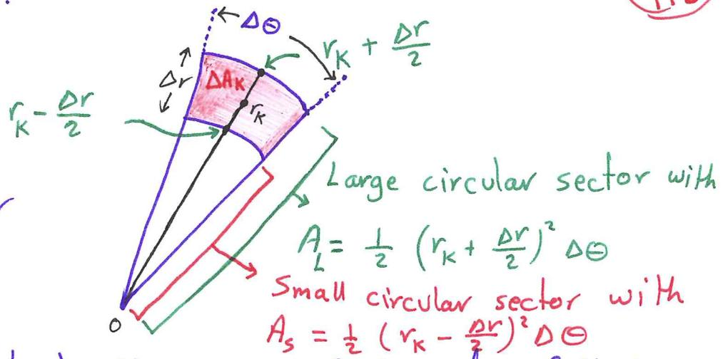
• We choose  $r_k$  to be the average of the radii of the inner and outer arcs bounding the  $k^{\text{th}}$  polar rectangle.
